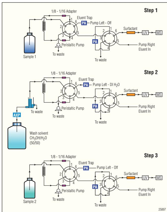
Figure 4. System schematic.
